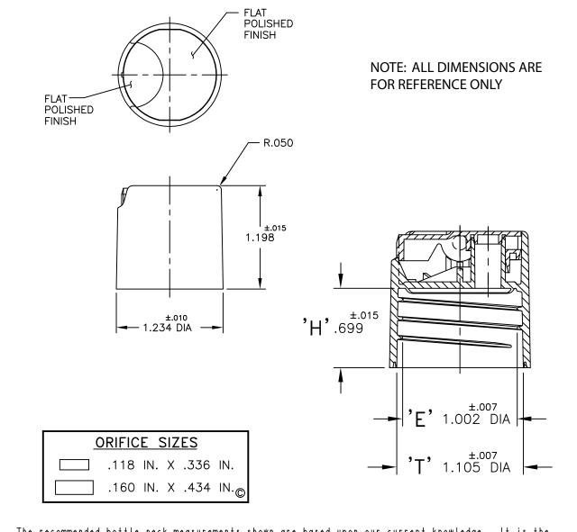
The recommended bottle neck measurements shown are based upon our current knowledge. It is the responsibility of the receiver of the information contained in these drawings to test for fit and function of the total package. Dimensions shown are intended for polyethylene bottles only. If another bottle material is used, some dimensions and tolerances may require adjustment.
