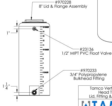
+970233 3/4" Polypropylene Bulkhead Fitting Tamco Vertical Closed Head Tank w/ Lid, Fitting & Float Valve
