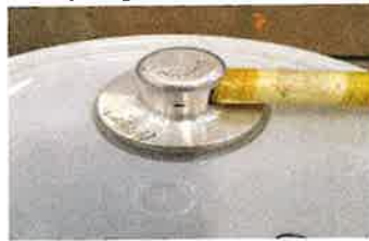
80 mm Screw Cap Tightened with torque wrench:
