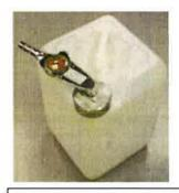
Step 4. Torque the cap to 240-270 in-lbs.
