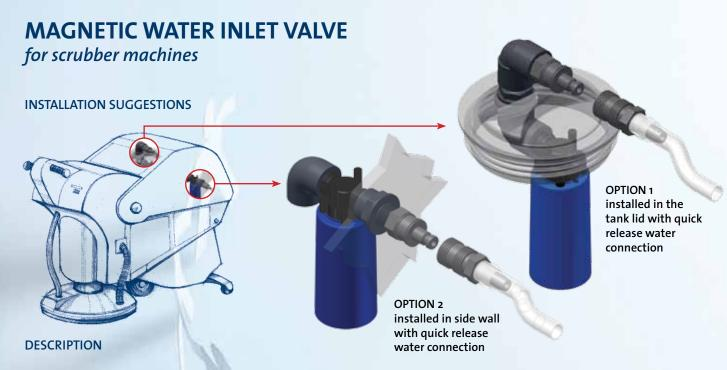
The Abertax Technologies Magnetic Water Inlet Valve features a float with an embedded magnet that will operate a diaphragm type valve. The rising water level lifts the float. The magnet inside the float then moves a stainless steel pilot plunger which closes the valve.
